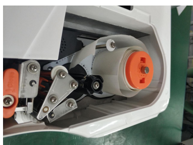
c. Open the print head module.
