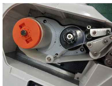
d. Tear off the first few pieces of label paper and send the paper across the rubber roller set.
